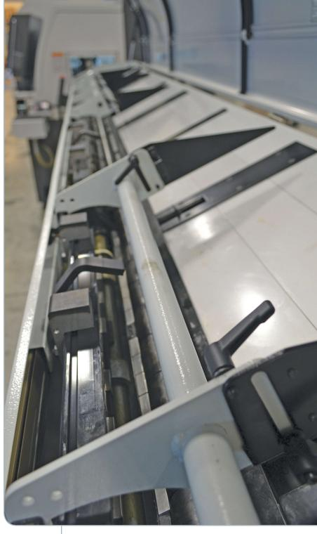
:: Magazine bar feeders hold multiple bars in reserve to extend the time a machine can run unattended.
